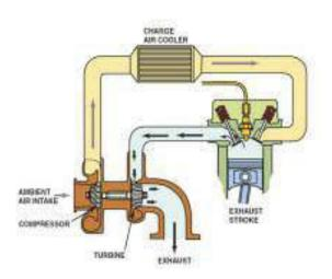
CAC range in size depending on the engine. They vary in sizes from smallest one for trucks/tractors & larger one for Marine applications.
